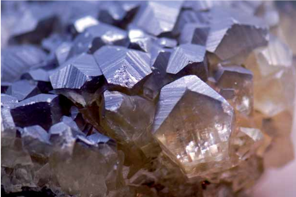
Quartz – base material for the silicate binder „water glass“ or „potassium silicate“
